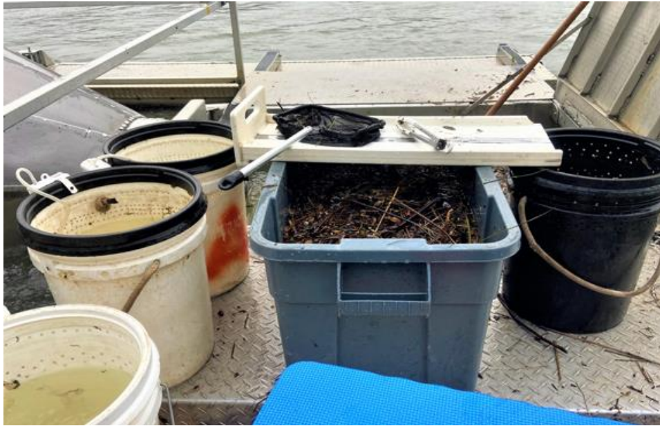
Figure 4: Trap work station, consisting of an 18-gallon tub, multiple 5-gallon holding buckets, a measuring board, and tongs.
